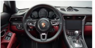
GT sports steering wheel with multifunction and steering wheel heating
